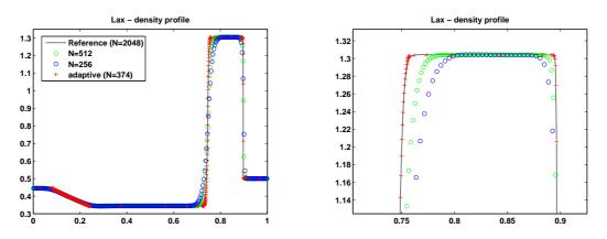
Figure 13: Lax problem with adaptive grid. Initial and minimum cell refinement level is 1, the maximum level is 11., i.e.,  $h_{\min} = 2^{-11}$ .  $S_{ref} = 10^{-3}$  was used in this run.
