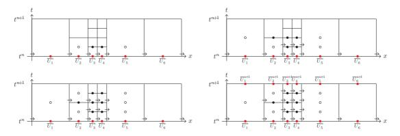
Figure 7: One timestep in CFL-mode for a grid with cells of 3 levels and a 1 stage Runge-Kutta.
