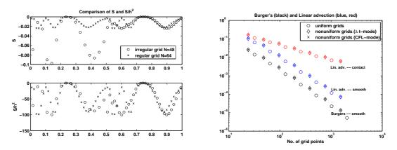
Figure 10: Left: entropy indicator for the transport of a sinusoidal wave. Right:  $L_1$  norm of the error on 3 tests with uniform meshes and non-uniform meshes.
