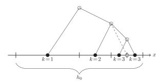
Figure 6: An example of diadic grid and its tree representation. On the rightmost cells, we show the tree representation of the refining/coarsening operation.
