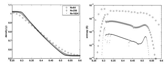
Figure 2: Euler equations, single left moving rarefaction wave. Solutions with different grid sizes (left) and entropy production in logarithmic scale (right).
