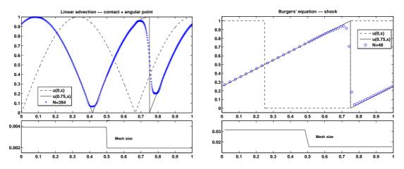
Figure 11: Solutions on non uniform meshes. Left: linear advection of a profile with a corner and a jump discontinuity. Right: shock on Burgers' equation.
