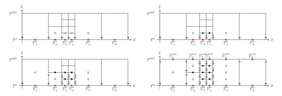
Figure 8: One timestep in CFL-mode for a grid with cells of 3 levels and a 2 stage Runge-Kutta.
