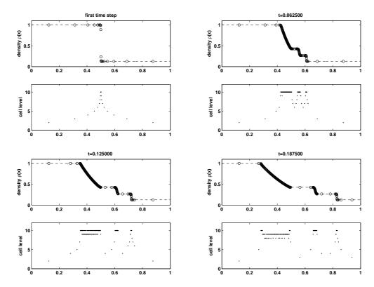
Figure 12: Sod problem with adaptive grid. Initial and minimum cell refinement level is 1, the maximum level is 10, i.e.,  $h_{\min} = 2^{-10}$ .  $S_{\text{ref}} = 10^{-3}$  was used in this run.
