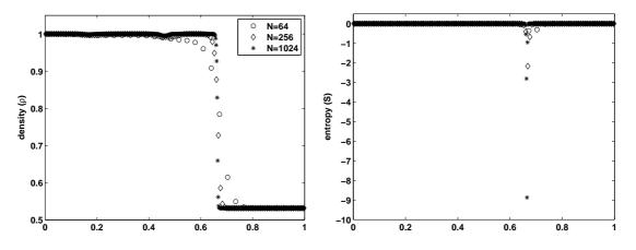
Figure 4: Euler equations, single right moving shock. Solutions with different grid sizes and entropy production.
